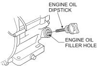
Figure 5. Oil Dipstick Removal
